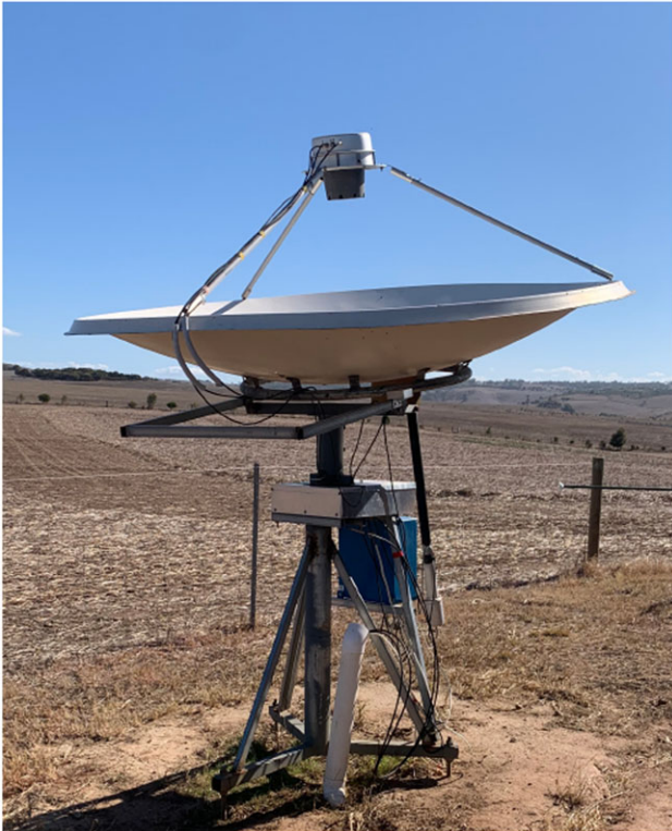
Figure 1. The 2.4 m Woodchester Observatory telescope. The dish is solid and has an f-ratio of 0.4. The receiver element is at prime focus and contains a ‘Clover-leaf’ dual-pole antenna of the type used at the UTMOST-NS project at the Molonglo Radio Telescope. It is protected by a black radome. The operating frequency of 820 MHz in a bandwidth of 8 MHz.
