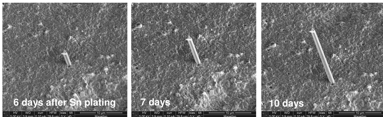
Fig. 1. SEM photomicrographs of Sn whisker growth. The tip morphology remains unchanged, with a so-called “cap grain” on top.
