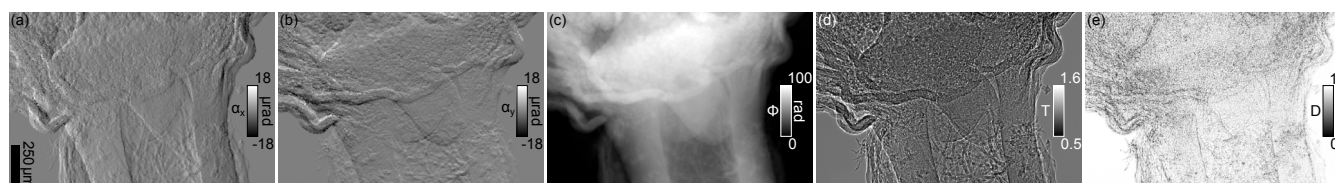
Figure 1. Multimodal signals of a flower bud obtained with UMPA: (a) Refraction angle in x , and (b) in y , (c) integrated phase, (d) transmission, (e) dark-field. Reprinted from [4], licensed under CC BY 4.0.
