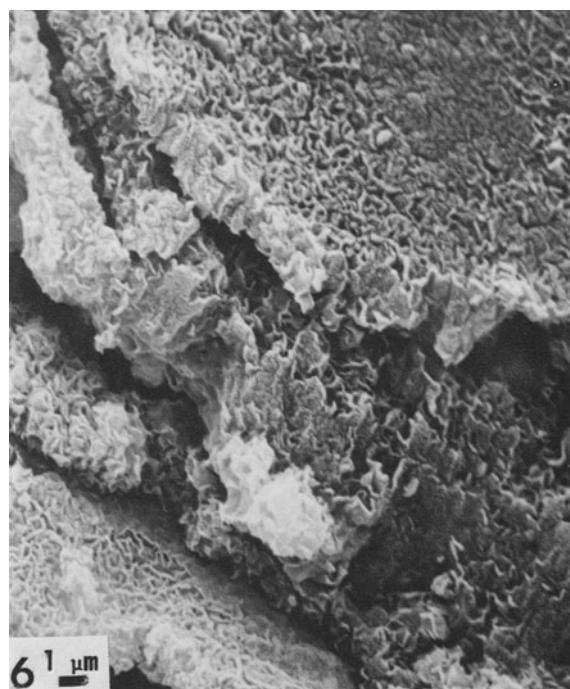
Figure 4. Scanning electron micrograph of sample API-26, Na-montmorillonite from Clay Spur, Wyoming, showing typical expanded, flared, "cornflake" or "oak leaf" texture of Na-montmorillonite; original instrument magnification = 6000 \times .
