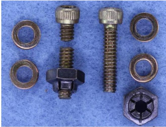
Figure 1. Broken cap screw and sister screw
