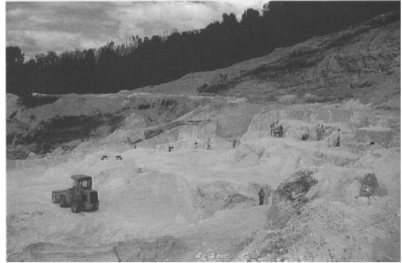
Figure 2. Lastarria open pit II (Afquintue) showing a white kaolinized quartz porphyry stock overlain by unaltered graphite-bearing micaschists.
