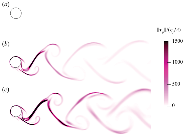
Figure 3. Normalized polymeric stress for different Weissenberg numbers: (a) Wi = 0.01 , (b) Wi = 4 , (c) Wi = 10 . For all these cases, other system parameters are kept constant at Re = 100 , U^* = 5 , A^* = 0.5 , L^2 = 10000 and \beta = 0.9 .
