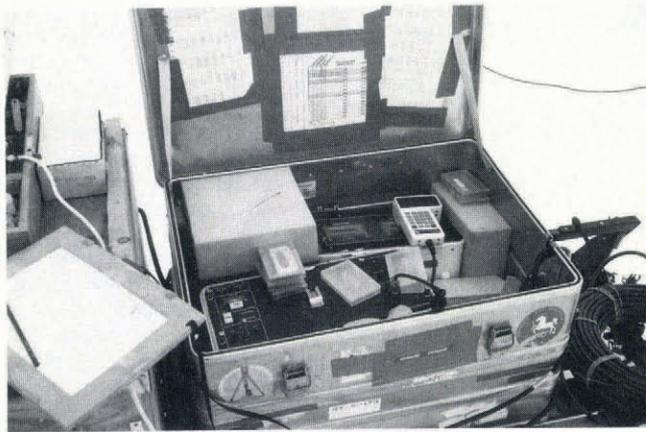
Fig. 4. TI4100 equipment: receiver/processor unit, control display unit, dual tape-drive recorder.
