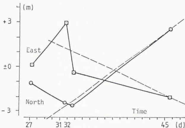
Fig. 10. Variation in local horizontal coordinates at station K53 (504) in 1987, from differential GPS.
