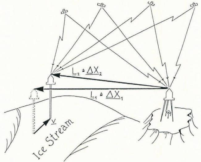
Fig. 5. The principle for ice-motion determination in the GPS differential mode.
