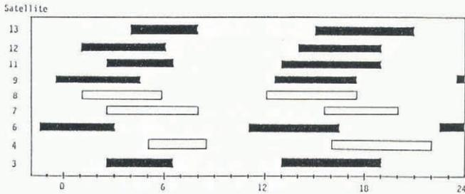
Fig. 2. Radio visibility of GPS satellites at Neumayer Station on 1 February 1987. Favorable observation conditions (four satellites) occurred between 14.00 and 18.00 GMT, dilution of precision occurred in the night coverage block. Satellites 4, 7 and 8 are not suitable for positioning.
