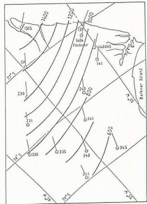
Fig. 9. Contour lines of the velocity and direction of ice-shelf motion in the area of Filchner Station in 1984. Partly preliminary results from on-line positions (Transit and GPS).
