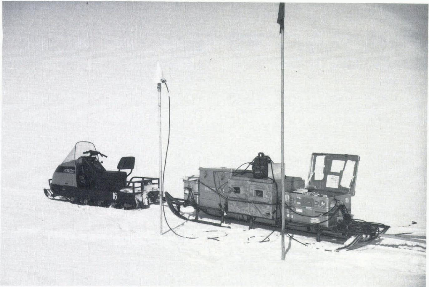
Fig. 3. TI 4100 receiver transport and measurement sled on Ekström Ice Shelf, 1987.
