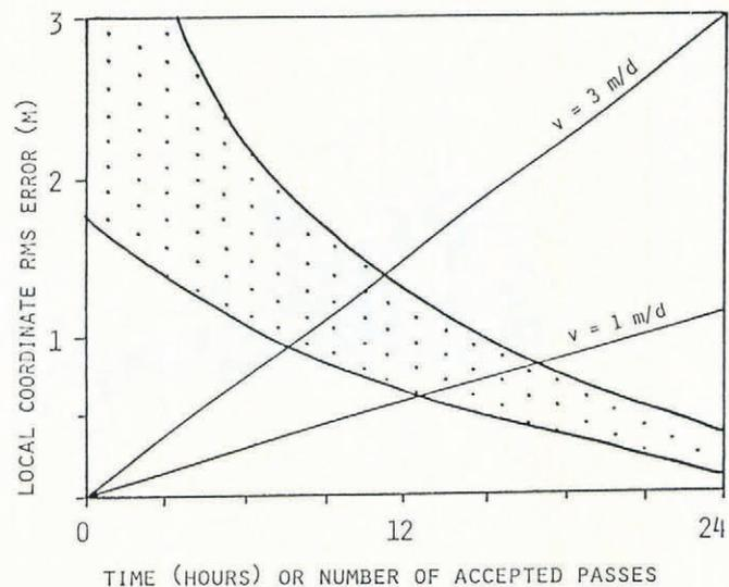
Fig. 6. Relation between coordinate error (Transit translocation) and station motion, assuming one pass per hour.
