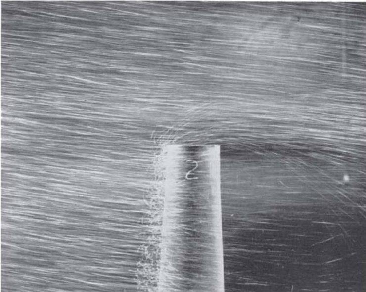
Fig. 3. Close-up photograph of unshielded gage showing air-flow pattern with blowing sawdust. [Note updrafts on left side of gage and the nearly horizontal path of particles as they pass over the orifice.] See text, p. 387
