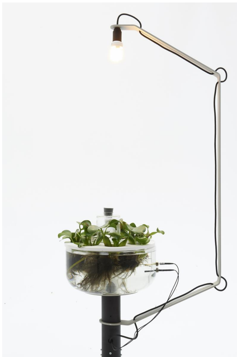
Figure 2. One of the three extraction units, featuring the ion selective electrodes immersed in the liquid ore.
