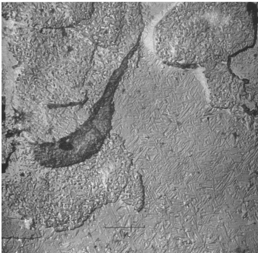
PLATE 1.—Electron micrograph showing oriented mullite needles after firing to 1300°C (17,300 ×).
