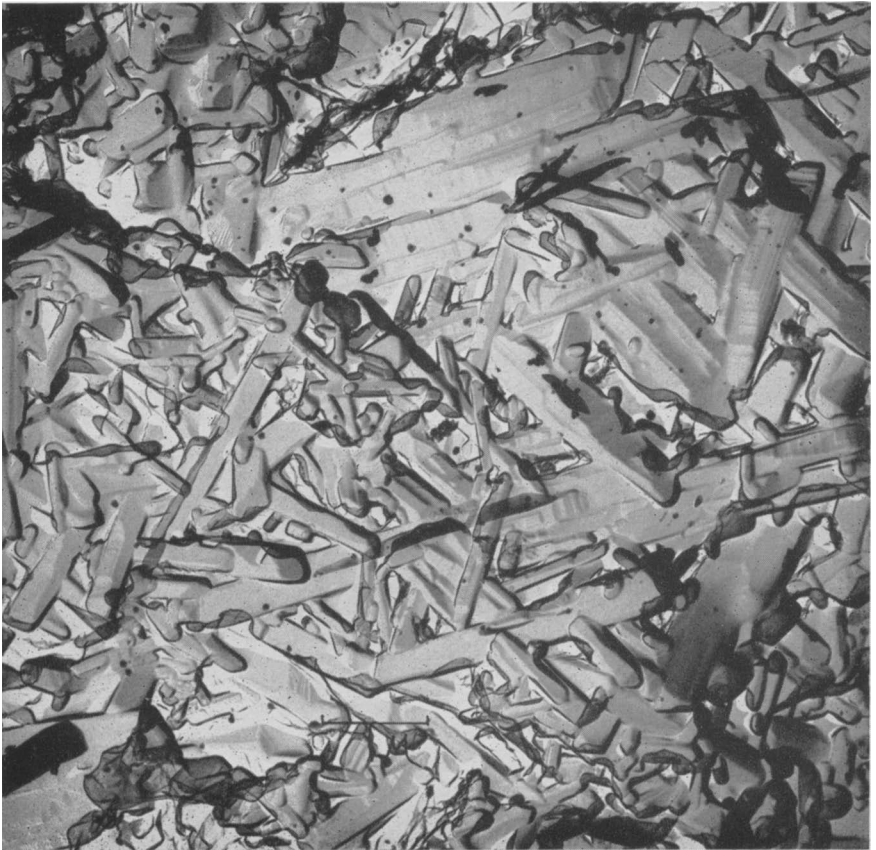
PLATE 2.—Mullite crystals developed from well-crystallized kaolin at 1400°C (13,800 ×).
