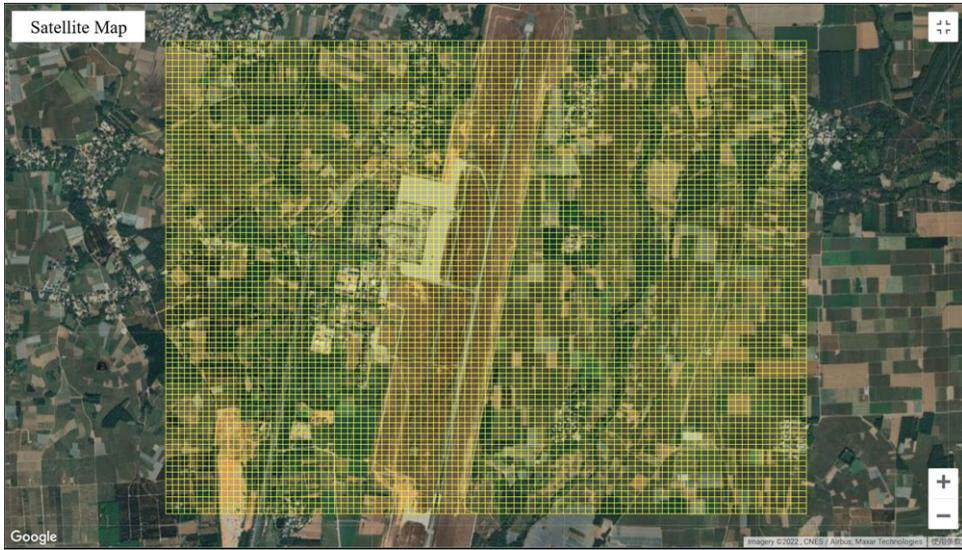
**Figure 2.** Spatial grid discretisation within radar surveillance airspace.
