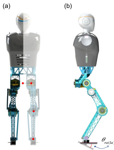
Figure 4. The leg geometry of the robot. The inverse kinematics solution is only for the four driving DoFs of the legs.
