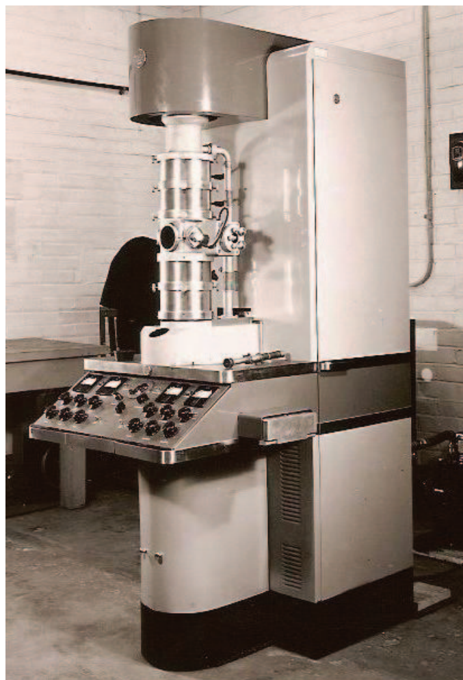
Figure 7: RCA model EMD-2 electron diffraction instrument.
