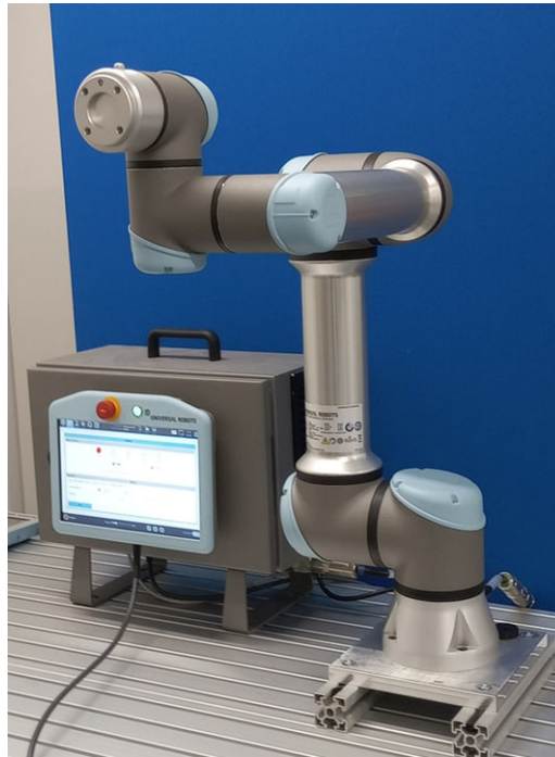
Figure 1. Experimental setup: the UR5e robot and its controller.
