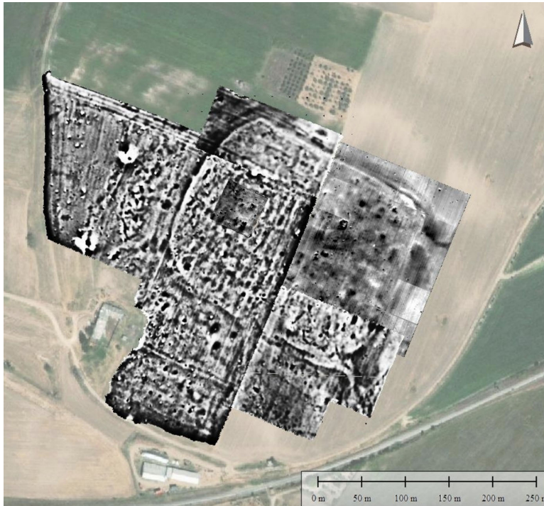
Fig. 2.32. Overview of the completed magnetometry survey at Toumba Serron. © BSA/Hellenic Ministry of Culture: Ephorate of Antiquities of Serres.
