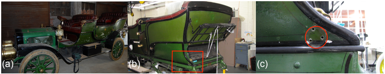
Figure 1. (a) White car prior to current conservation workshop at The Henry Ford Museum. (b) Rear view of vehicle with one area from which paint was sampled outlined in red. (c) Paint sample for microanalysis removed from region outlined by red circle.
