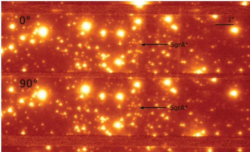
**Figure 1.** The arrangement of the Wollaston prism images on the NACO detector. The two central strips show the images in orthogonally polarized light.
