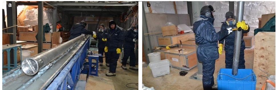
Fig. 5. (a) Filter for cuttings and (b) emptying cuttings from the filtering tool.
