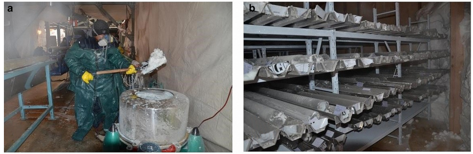
Fig. 4. (a) Centrifuging fluid from the cuttings and (b) ice cores in the ice storage room.
