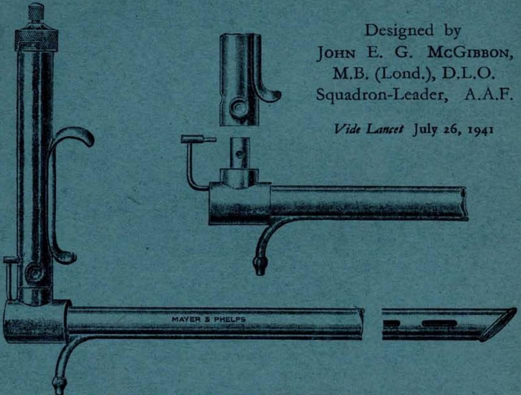
A Bronchoscope self contained with battery in handle, dispensing with entangling cables.
