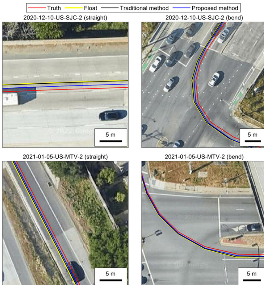
Figure 8. Typical positioning performances on the map of the truth, float, traditional and proposed method solutions of straight and bend conditions.
