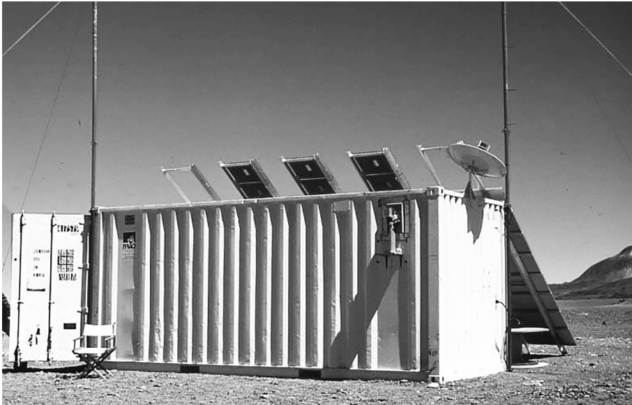
Figure 4.10 The atmospheric monitoring laboratory in the center of the Chajnantor site. It was built into a standard shipping container. The array of solar panels leaning on the back side of the container provided power. The tipping mirror mechanism of the 225 GHz radiometer can be seen mounted on the top right-hand side of the container. The small antenna on the end of the container provided a data connection via SatPhone. Credit: Paul Vanden Bout; NRAO/AUI/NSF, CC BY 3.0.
