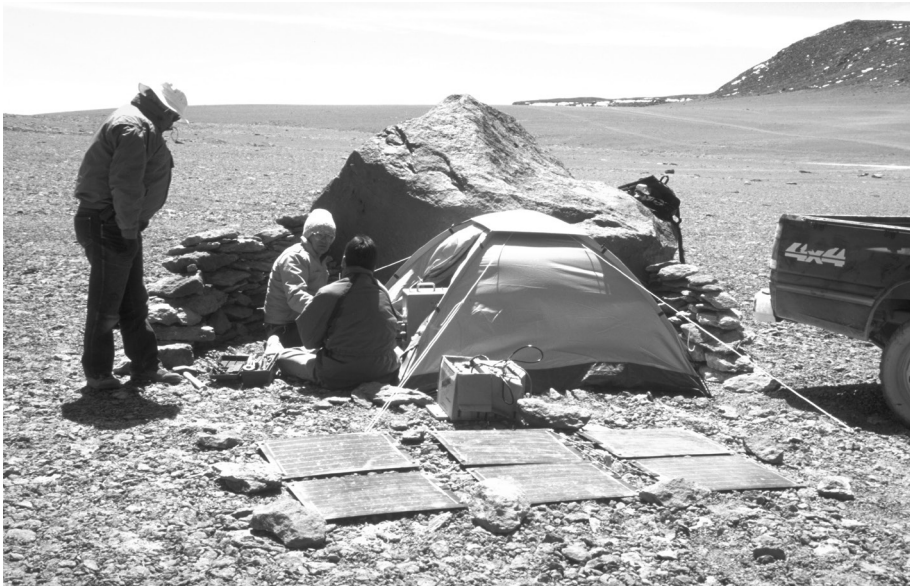
Figure 4.9 The first MMA site survey team and their equipment: tipping radiometer in the entrance to the tent and solar panels for charging the batteries that powered the tipper in front. Left to right: Peter Napier, Frazer Owen, and Angel Otárola. Credit: Simon Radford; NRAO/AUI/NSF, CC BY 3.0
