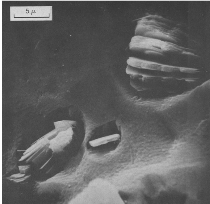
Fig. 5(a). Normal view of pyrite cleat surface with kaolinite packets growing through; Herrin (No. 6) Coal Member, Carbondale Formation, Sangamon Co., Illinois (Pennsylvanian).
