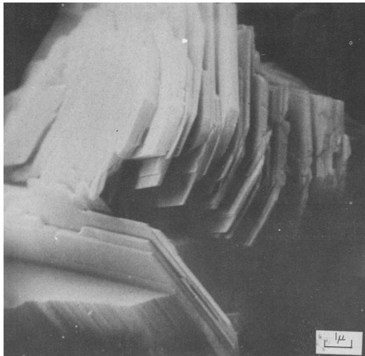
Fig. 14(b). Cantilevered stacking sequence of platelets in kaolinite stack; concretion in Francis Creek Member, Carbondale Formation, Grundy Co., Illinois (Pennsylvanian).
