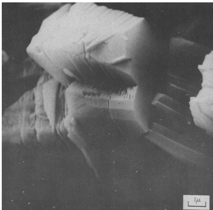
Fig. 3(b). Authigenic cleat kaolinite from the Herrin (No. 6) Coal Member, Carbondale Formation, Sangamon Co., Illinois (Pennsylvanian).
