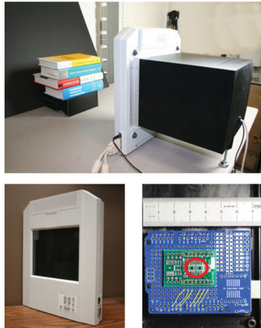
Fig. 7. Prototype device. Top: lab setup. Bottom left: the LCD screen as the aperture assembly. Bottom right: the sensor board with two sensors, indicated by the red circle.
