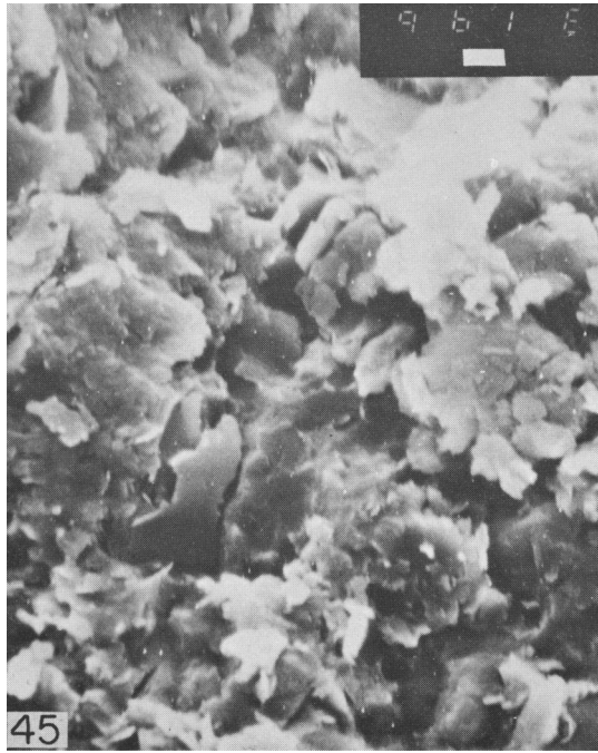
Figure 45. SEM, at 6000 \times , of highest quality flint clay, underground mine at Iwate. Angularity of crystal edges and individual crystal plates attest to recrystallization of kaolin, presumably during structural tilting of the rocks, 3196.
