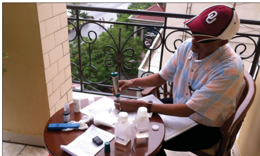
Graduate student Teshome Yami tests fluoride concentration in water in a makeshift laboratory in Ethiopia. His work is part of a USAID project where researchers from Addis Ababa University and The University of Oklahoma are developing affordable aluminum-based materials to remove fluoride from potable water. Credit: Teshome Yami.
