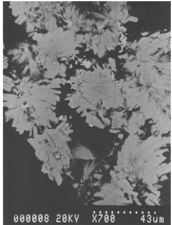
Figure 10. Mordenite is formed at the expense of heulandite minerals in the tuff's matrix.
