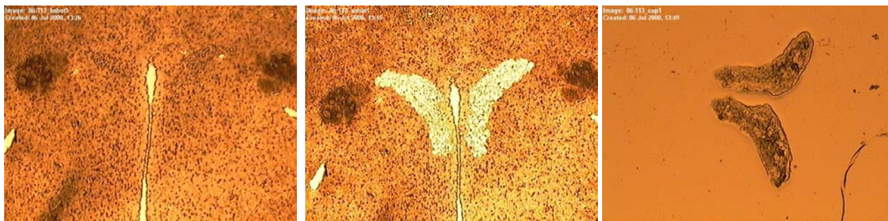
Figure 1. Laser capture microscopy dissection of the paraventricular nucleus from mouse brain. Sections were used to quantify total RNA yields correlating to the orphan GPCRs after primer amplification.
