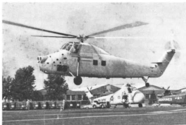
Fig 2 Twin Turbine version of the Sikorsky S 58
