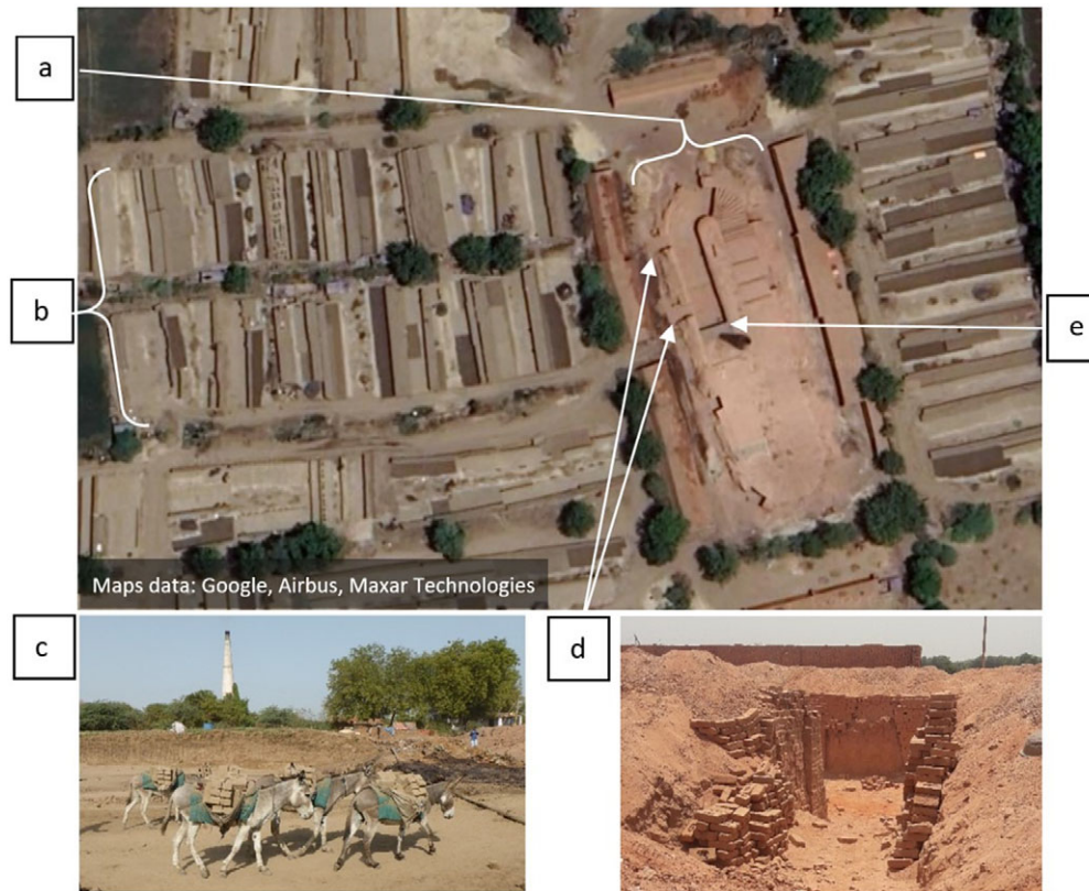
Figure 1. An example brick-kiln site visited during fieldwork in Gujarat, India, during May 2018, to demonstrate the movement of donkeys during brick transportation into the kiln (a). Showing wet bricks moulded and stacked in rows (b), where they are loaded into pack saddled carried by donkeys (c). Donkeys and their owners then walk to a kiln entrance (d), and through to where the bricks are offloaded and stacked within the kiln (e), ready to be covered and fired once the kiln is full. (Photo credit (c, d): LM Kubasiewicz).
