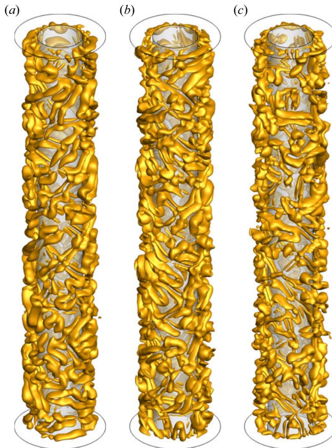
Figure 23. The 3-D vortical structures for (a) V_E = 4000 ( Q=20 ), (b) V_E = 5000 ( Q=30 ) and (c) V_E = 6000 ( Q=30 ) (see supplementary movies 18 and 19).
