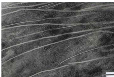
FIG. 1. Electron micrograph showing a section of 1%LPE blend after chlorosulphonation. Microscale represents 0.1 \mu\text{m} .
