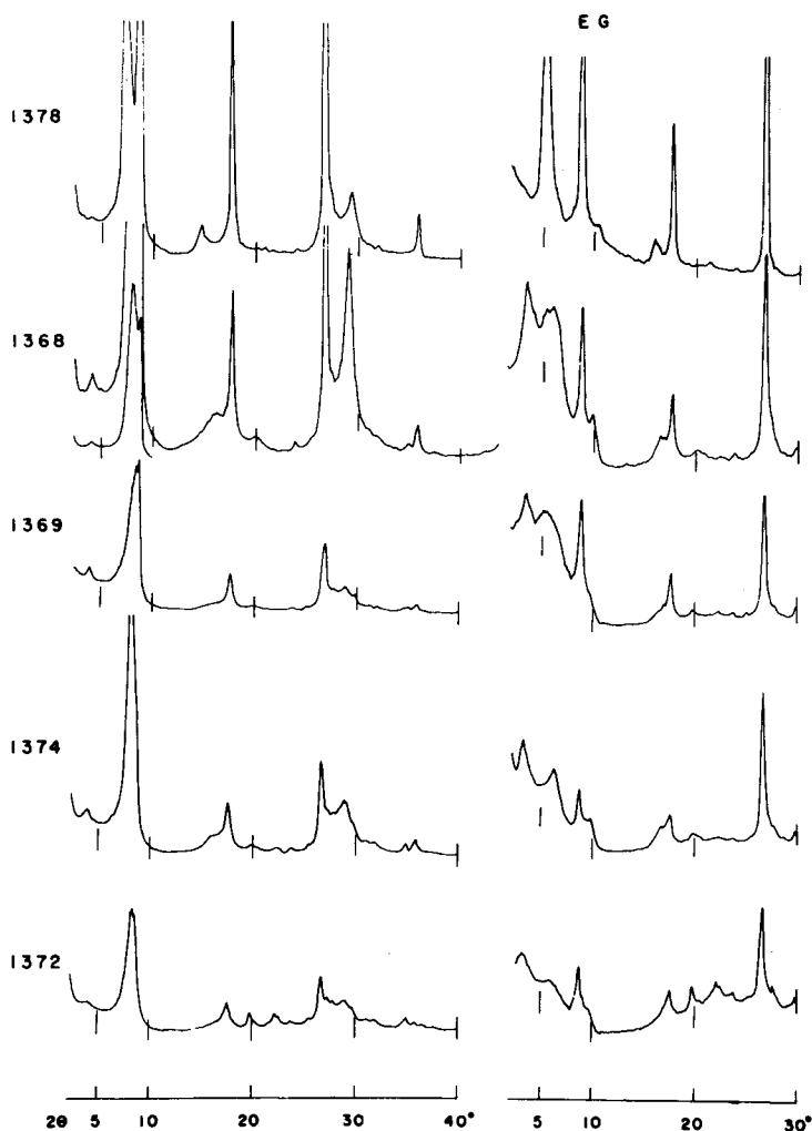
Fig. 2. X-ray diffraction patterns of specimens formed from various compositions after 75 hr reaction. 1378, sericite(0.2 g) + \text{LiNO}_3 (2 g) + \text{NaCl} (0.005 g); 1368, sericite(0.2 g) + \text{LiNO}_3 (2 g) + \text{NaCl} (0.01 g); 1369, sericite(0.2 g) + \text{LiNO}_3 (2 g) + \text{NaCl} (0.02 g); 1374, sericite(0.2 g) + \text{LiNO}_3 (2 g) + \text{NaCl} (0.025 g); 1372, sericite(0.2 g) + \text{LiNO}_3 (2 g) + \text{NaCl} (0.04 g).
