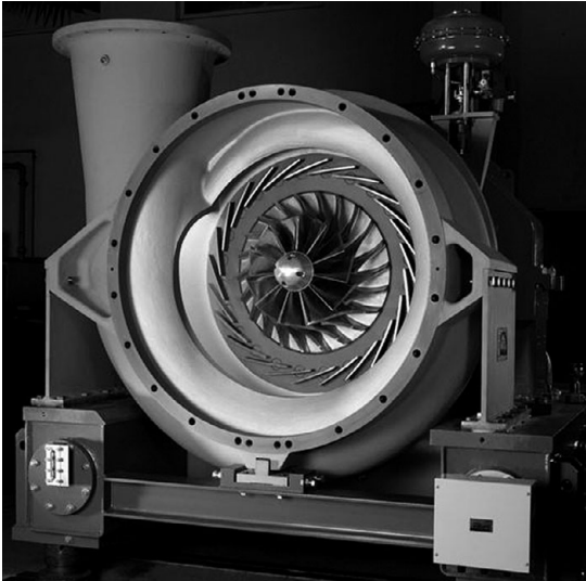
Figure 1.8 A single-stage compressor with a variable vaned diffuser and a volute with the inlet casing removed. (image courtesy of MAN Energy Solutions)
