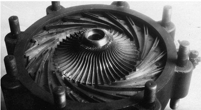
Figure 1.18 An impeller and diffuser from a radial compressor stage of the 1904 gas turbine of Aegidius Elling. (image by Aegidius Elling courtesy of the Norway Museum of Science and Technology)
