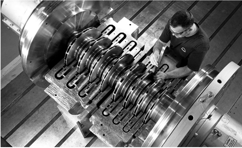
Figure 1.24 A barrel compressor showing the horizontally split internals extracted from the barrel casing. (image courtesy of MAN Energy Solutions)
