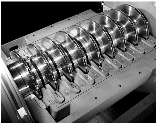
Figure 1.9 A nine-stage compressor with shrouded impellers. (image courtesy of MAN Energy Solutions)
