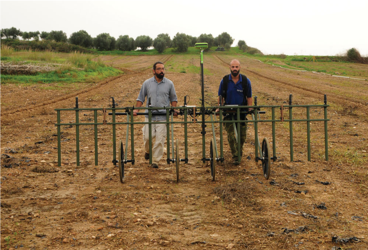
A Sensys multi-sensor gradiometer from the Institute for Mediterranean Studies in use at the classical Greek city of Elis. This survey has mapped an extensive road network to the east, south and west of the central agora of this important city, well known for serving as the administrator for the ancient Olympic Games. The survey was undertaken as part of the AncientCity project which is investigating the use of geophysical and remote sensing methods on sites in the Peloponnese and Central Greece. (c) Ian Moffat.
