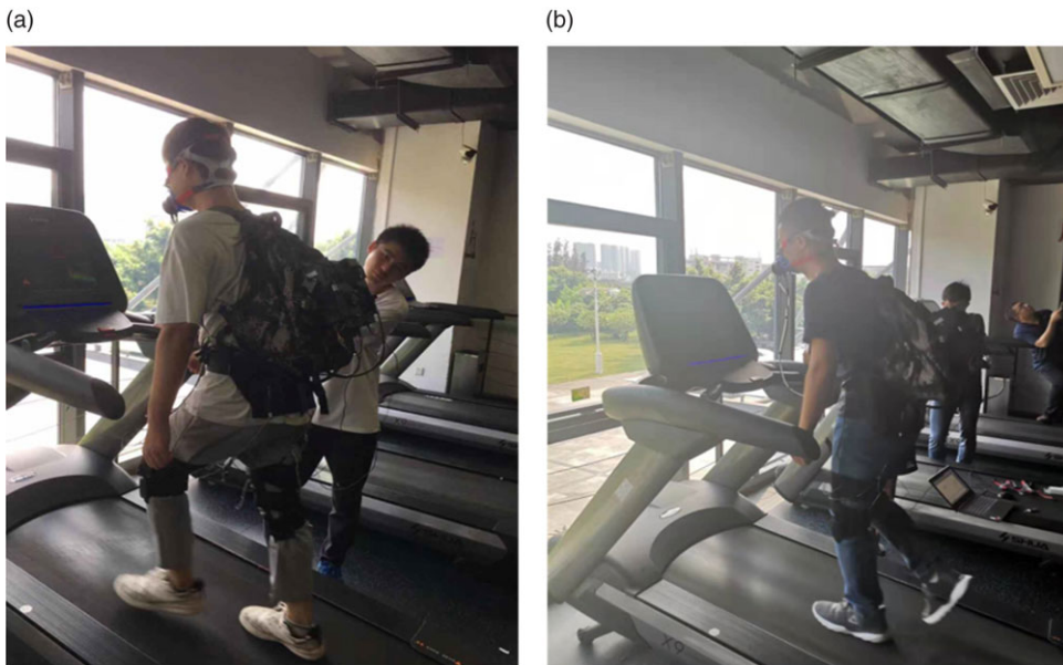
Figure 5. Some participants carry K5 on a treadmill with a load of 25 kg and walk at an average speed of 5 km/h.
