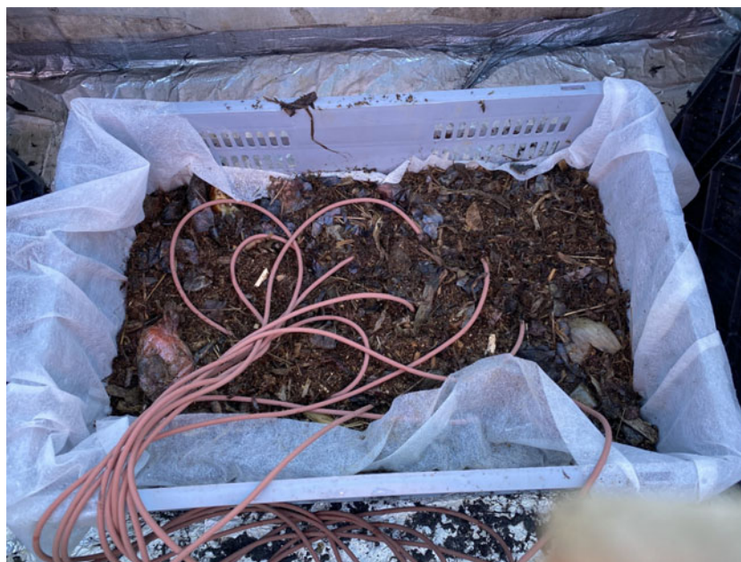
Figure 1. Box with compost consisting of onion waste (60%), horse manure (20%), and wood shavings (20%) and thermocouples mounted at different places in the box.
