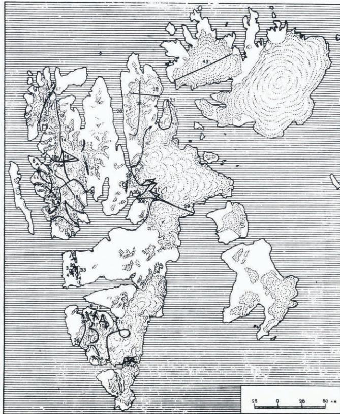
Fig. 3. Radio echo-sounding of the Svalbard glaciers during 1974–75 and 1977–79. Lines show the routes of the airborne radio echo-sounding. Mountain glaciers: 1—Aldegondabreen, 2—Vøringbreen, 3—Dahlfonna, 4—Erdmannbreen, 5—Austre Brøggerbreen, 6—Vestre Brøggerbreen, 7—Midre Lovénbreen, 8—Antoniabreen, 9—Hessbreen, 10—Penckbreen, with tributaries Suessbreen and Tjolarbreen (in the east), 11—Sveisarfonna, 12—Finsterwalderbreen with tributaries Revtannbreen (in the west) and Leinbreen (in the east), 70—Bertilbreen; “reticulated” glaciers: 13—Monacobreen, 14—Isachsenfonna, 15a—Kongsbreen, 15b—Kronebreen, 16—Holtedahlfonna, 17—Kongsvegen, 18—Sveabreen, 19—Dahlbreen, 20—Konowbreen, 21—Aavatsmarkbreen, 22—Uversbreen, 23—Løvenskioldfonna, 24—Åsgårdfonna, 25—Valhallfonna, 26—Sorobreen, 27—Lomonosovfonna, 28—Mittag-Lefflerbreen, 29—Negribreen, 30—Nordenskiöldbreen, northern (a) and southern (b) flows; 31—Tunabreen, 32—Vestre Grønfjordbreen, 33—Austre Grønfjordbreen, 34—Fridtjovbreen, 35—Recherchebreen, 36—Vestre Torellbreen, 37—Austre Torellbreen, 38—Hansbreen, 39—Hornbreen, 40—Hambergbreen, 41—Samarinbreen, 42—Olsokbreen, 44—Odinjøkulen, 45—Torsfonna, 46—Balderfonna, 47—Kantbreen, 48—Veteranen, 49—Månebreen, 50—Stubendorfbreen, 51—Cookbreen, 52—Elnabreen, 53—Orsabreen, 54—Sefstrømbreen, 55—Holmstrømbreen, 56—Osbornebreen, 57—Wahlenbergbreen, 58—Borebreen, 59—Nansenbreen, 60—Eidembreen, 61—Løvliebreen, 62—Vestgotabreen, 63—Holmesletbreen, 64—Skipperbreen, 65—Hydrografbreen, 66—Comfortlessbreen, 67—Idabreen, 68—Raudfjordbreen, 69—Lilliehøkbreen, 71—Werenskiöldbreen, 72—Vrangpeisbreen, 73—Amundsenisen, 74—Høgstebreen, 75—Bjørnbreen, 76—Nathorstbreen, 77—Ljosfonna, 78—Dobrowolskibreen, 79—Pollakbreen, 80—Muhlbacherbreen, 81—Opalbreen; ice sheets: 43—Vestfonna (Nordaustlandet). Types of the glaciers are given in accordance with classification derived from the work by Troitskiy and others (1975).
