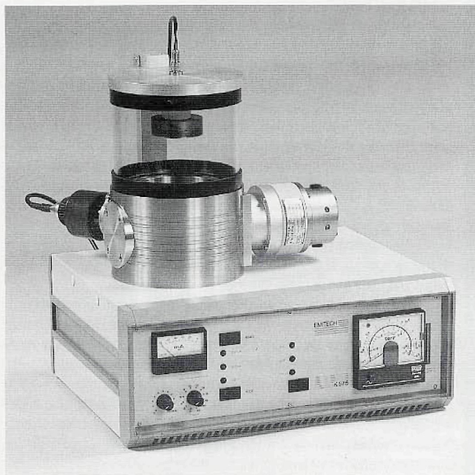
K575 (illustrated) Turbo Pumped Sputter Coater for Chromium K550 Sputter Coater for Gold K650 Large Sample Sputter Coater
