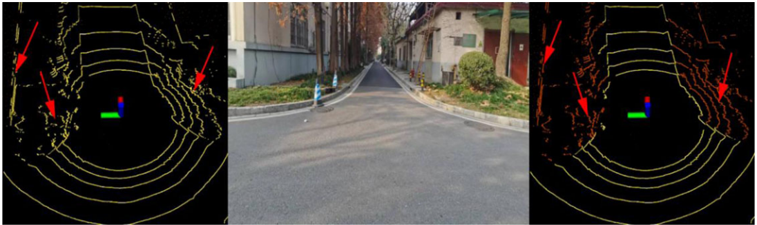
Figure 5. A scene of downhill (The LeGO-LOAM segmentation algorithm is on the left side, and our method is on the right side).
