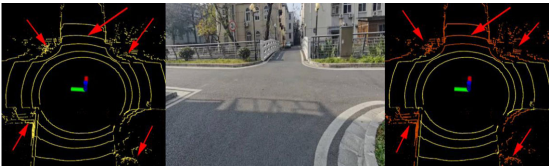
Figure 4. A scene of uphill (the left picture is obtained by the LeGO-LOAM segmentation algorithm, and the right picture is obtained by the method proposed in this paper. The yellow dots are considered ground points).
