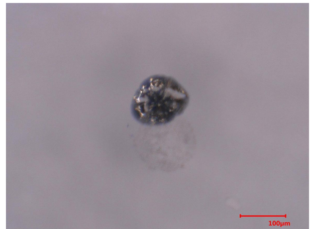
Figure 6. The damage spot micrograph of the GaN single crystal specimen (the measuring scale is shown in the figure).
