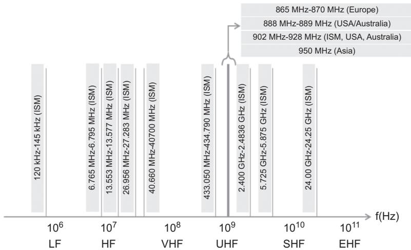
**Figure 2.2** Available worldwide frequency bands for RFID.
