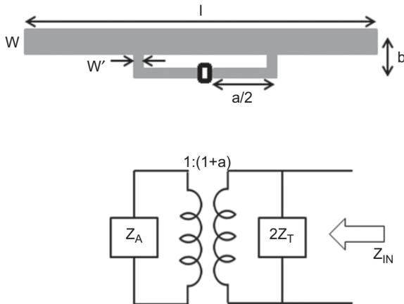
**Figure 2.6** The T-match structure and the equivalent circuit.
