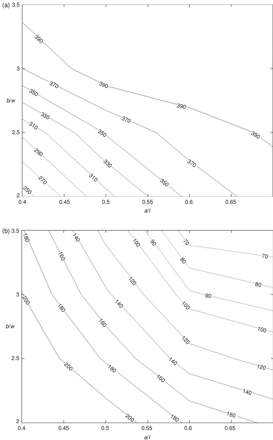
**Figure 2.7** The T-match structure matching chart for the case of  $l = \lambda/2$ ,  $w = \lambda/100$ ,  $w' = w/2$ , (a) resistance ( $\Omega$ ) (b) reactance ( $\Omega$ ).
