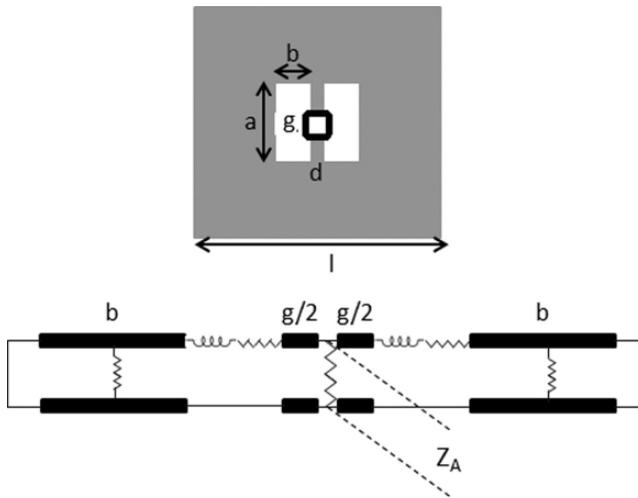
**Figure 2.10** The nested-slot structure and the equivalent circuit.
