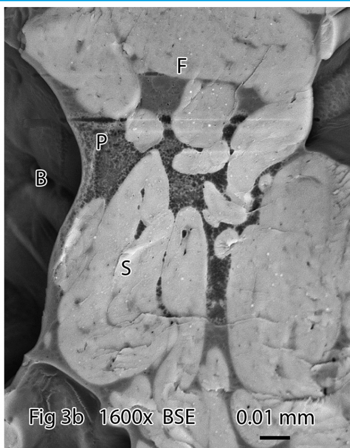
Fig 3 a,b Sectioned whey crisps stained with iodine. 1600 × magnification BSE mode. B = bubble, F = fractured face of crisp, P = protein-rich region, S = starch-rich region.
