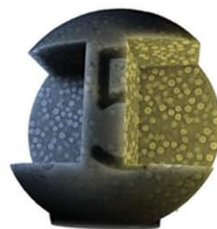
Pharmaceutical tablet at 14.4 mm FOV with Mo radiation
