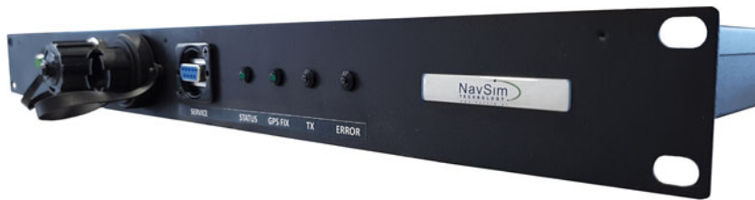
Figure 3. Virtual AtoN generator (front view, 19-inch rack mount).
