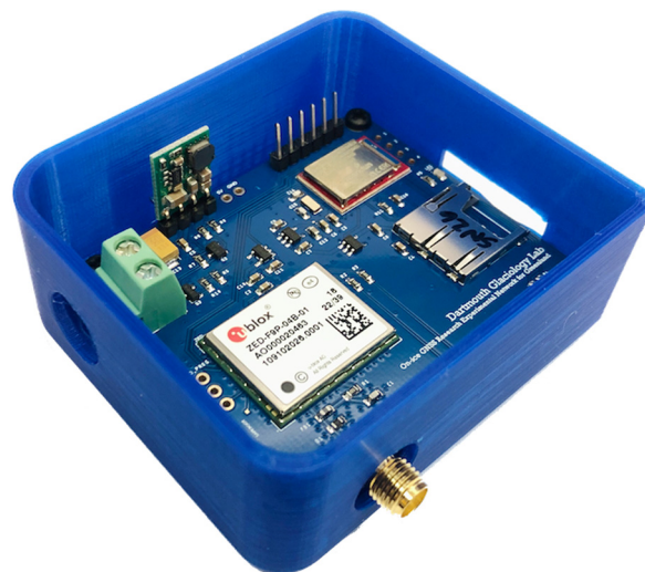
Figure 1. OGRE in 6.75 \times 6 \times 2.75 cm 3D-printed housing with lid removed. For field applications, we place this assembly inside a waterproof housing with bulkhead connections to the antenna and battery.
