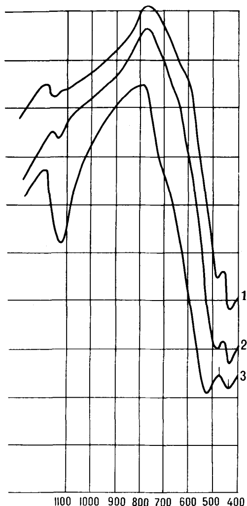
Figure 5. Infrared spectra of rancieite from the Urals (1 = sample 1, 2 = sample 2) and the birnessite from the Pacific Ocean (3 = sample 3). Abscissa in \text{cm}^{-1} .
