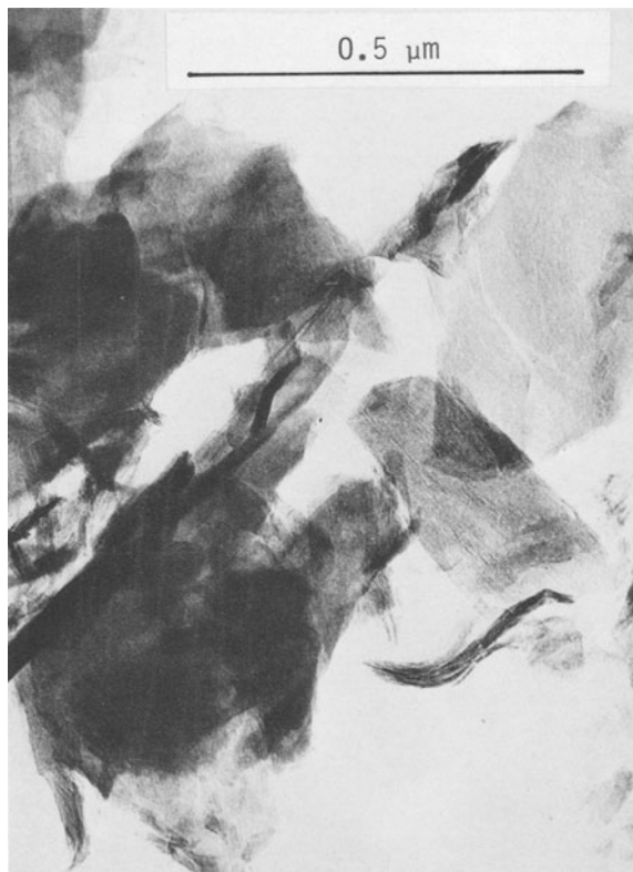
Figure 3. Transmission electron micrograph of birnessite from the Chiatura deposit in Georgia.
