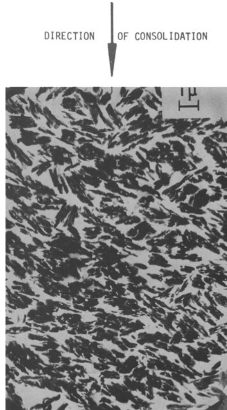
Fig. 3. Electron-micrograph of thin section of 900 Å through kaolinite impregnated with Araldite AZ15, consolidated from 150 per cent moisture content, pH8, under 4.75 Kg/cm 2 . (Soft material).
