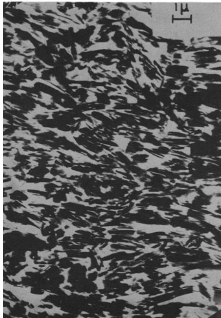
Fig. 4. Electron-micrograph of thin section of 900 Å through kaolinite impregnated with Araldite AZ15, consolidated from 500 per cent moisture content, pH8, under 45 Kg/cm 2 . (Hard material).
