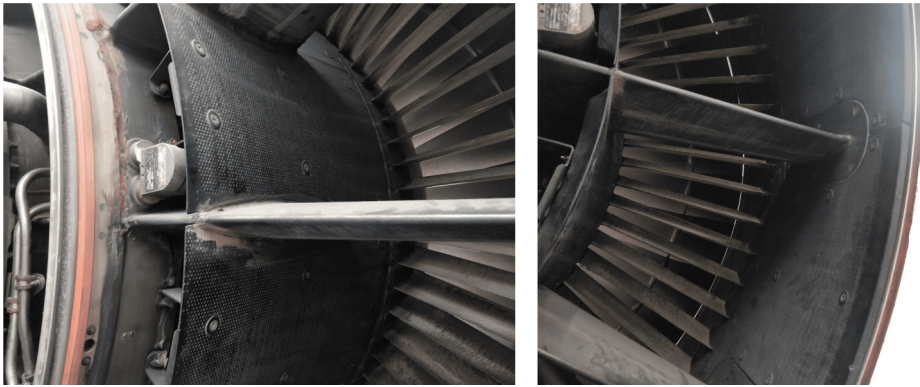
Figure 2. Acoustic liners around the fan of a turbofan engine.
