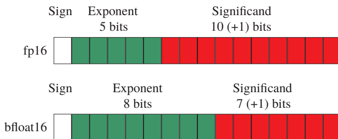
Figure 2.1. Comparison of the 16-bit bfloat16 and fp16 floating-point number formats. The ‘+1’ refers to the implicit leading bit of the significand, which is not stored.
